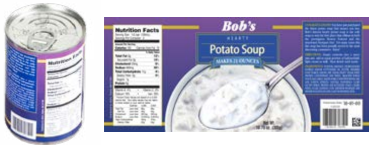
Figure 3: A line scan camera unwraps the curved surface of a rotating can to capture its label without image distortion.
